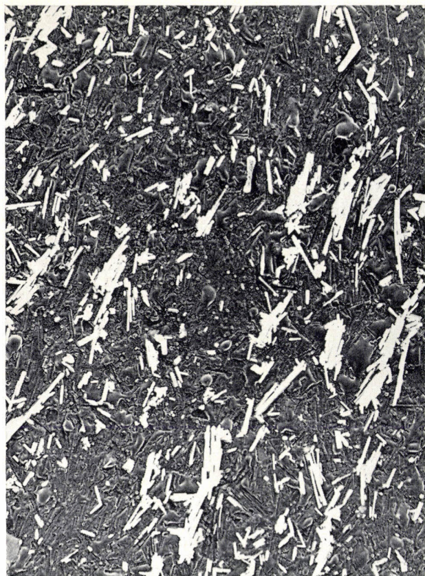
Fig. 7. Electron photomicrographs of the magnetic layer of a ) a tape with cubic iron-oxide particles, in common use about 20 years ago; b ) a tape with needle-shaped iron-oxide particles as commonly used today, and c ) a recently marketed tape with chromium-dioxide particles. The magnification of all three photomicrographs is 14\,500\times . Those in ( b ) and ( c ) were made by the replica technique; in ( c ) the white bars are chromium-dioxide needles that have stuck to the replica, while other chromium-dioxide needles have only left impressions in the replica.
